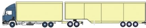
Type 3: Trucks with a lower axle and semi-trailer (maximum length of 25.25 m)
